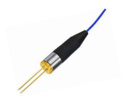
The FCML series diode lasers deliver up to 50mW of power through a 50/125µm fiber. They feature built-in optical isolator, low capacitance and low dark current, high stability, low threshold current, low operating current, integrated high isolation, and low insertion loss.
